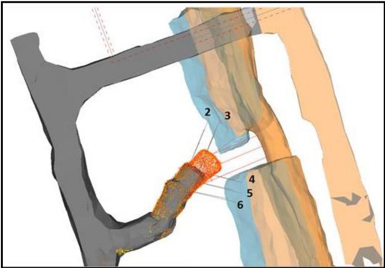
Figure 3. Location of the sections on the sides of the cross-member
