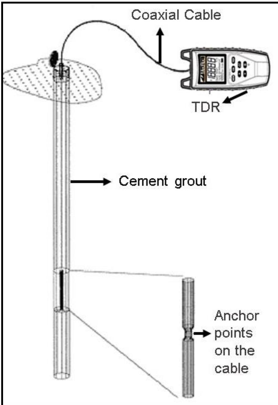
Figure 1. Characteristics of the TDR installation showing the relationship between cable and instrumentation
