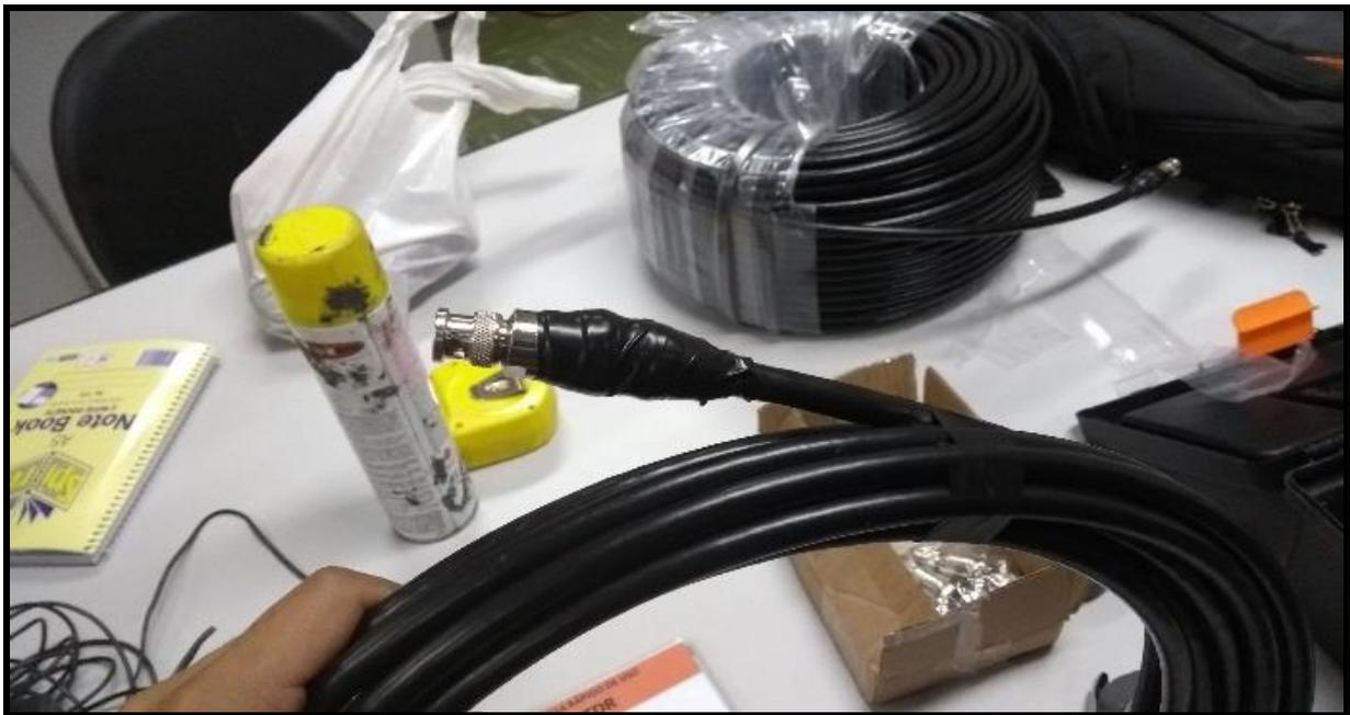
Figure 7. BNC conector installed on the cable
