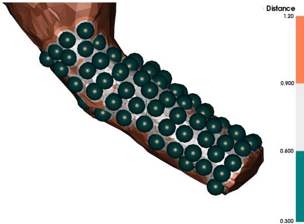
Fig. 6 - Bolt pattern of the Pequizão mine.
