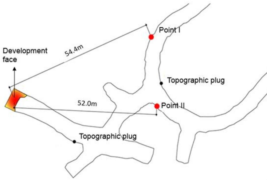
Figure 2. Location of monitoring points at a development blasting
