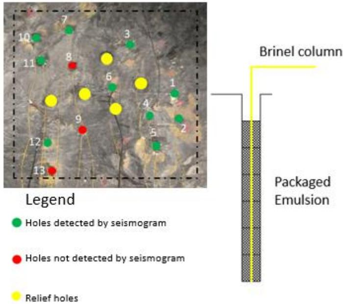
Figure 4. Slot blasting sketch (left) and charging components into the holes (right)
