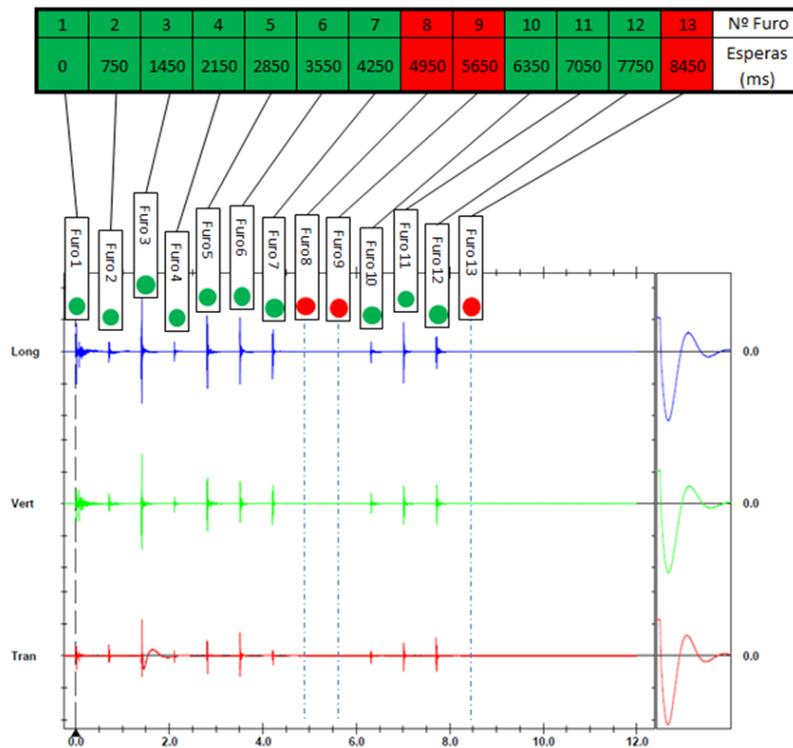
Figure 3. Seismogram of one confined mining blasting
