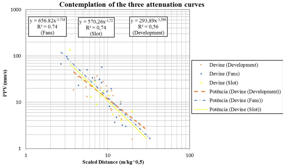
Figure 6. Attenuation curve for each type of blasting operation
