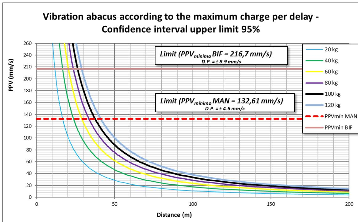
Figure 7. Vibration abacus according to the maximum charge per delay - Confidence interval upper limit 95%
