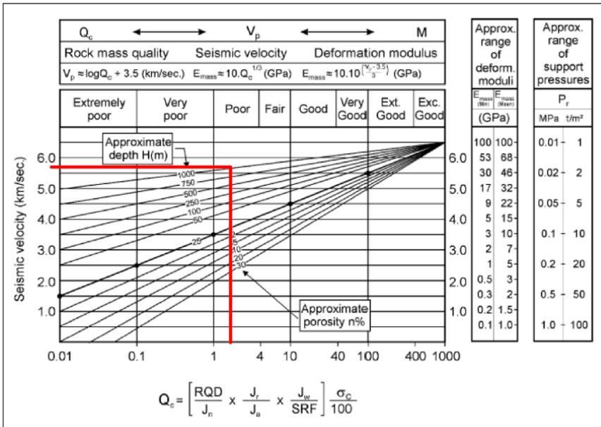
Figure 5. Barton Abacus - Definition of Vp (wave propagation velocity), according to depth and quality of rock mass "Q".
