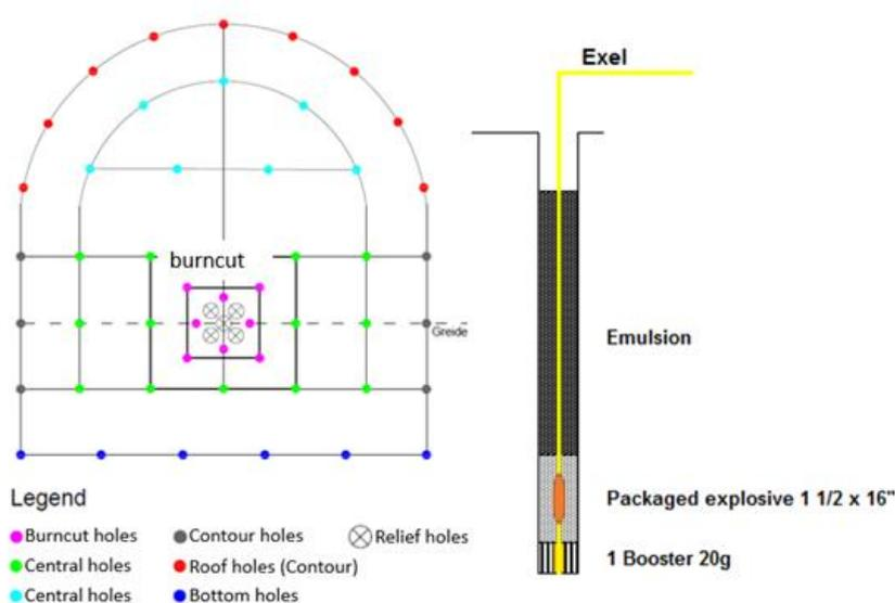
Figure 1. Development section (left) and charging components into the hole (right)
